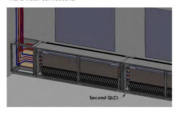
b.) Connect the QLCI units together by sliding the connector sleeve from the adjacent QLCI unit onto the entry spigot and seal the connection as described below in **Section 3.5.**
