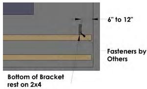
b.) Hang the lower Fin Tube Elements by placing them gently onto the Fin Tube Mounting Brackets. The tubes of the Fin Tube Elements will rest in the V-Groove of the Fin Tube Mounting Brackets. The Fin Tube Elements are 2.75" fin width and 2.50" fin height. Make sure the Fin Tube Elements are positioned in the correct orientation.
