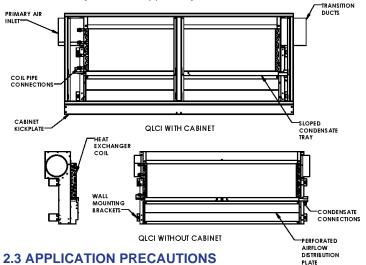
When in cooling mode, the entering water temperature to the QLCI displacement induction ventilation diffuser coil should be maintained warmer than the space dew point temperature in order to prevent condensation.
