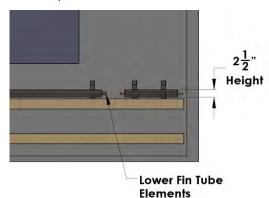
c.) Hang the upper Fin Tube Elements by placing them gently onto the Fin Tube Mounting Brackets. The tubes of the Fin Tube Elements will rest in the V-Groove of the Fin Tube Mounting Brackets. The Fin Tube Elements are 2.75" fin width and 2.50" fin height. Make sure the Fin Tube Elements are positioned in the correct orientation.
