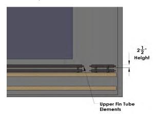
d.) Repeat Steps (a-c) for additional Fin Tube Elements according to the room layout of the project plans. Note: There may be plastic clips on the Fin Tube Elements from the manufacture, these can be discarded.
