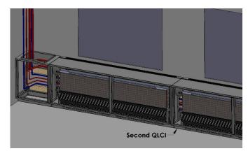
b.) Connect the QLCI units together by sliding the connector sleeve from the adjacent QLCI unit onto the entry spigot and seal the connection as described below in **Section 3.5.**
