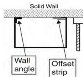
The cover is field mounted (by others) using painted countersunk screws (provided) per wall attachment angle.
