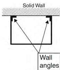
The cover is field mounted (by others) using painted countersunk screws (provided) per wall attachment angle.
