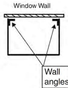
The cover is field mounted (by others) using painted countersunk screws (provided) per wall attachment angle.
