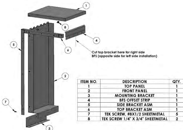
**The preferred method of cutting the parts is to use a bench or floor mounted metal cutting bandsaw.** Alternative equipment to use is either a 90deg cutting wheel or die grinder to make the cuts. Deburr sharp edges once cuts are complete. The side and top brackets that cover the top and front panels have 7/8" of overlap to cover the cut edges.
