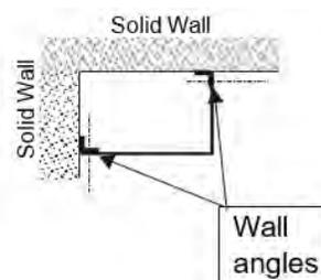
The cover is field mounted (by others) using painted countersunk screws (provided) per wall attachment angle.
