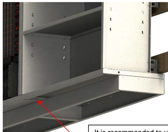
It is recommended to use these holes on the BBS/ DBS top and bottom panels to attach each unit together.
