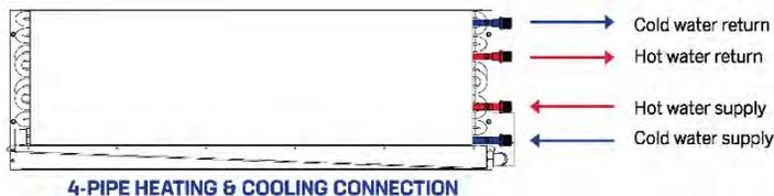
Piping should be insulated and properly labeled in accordance with local building codes, similar to what is shown below.
